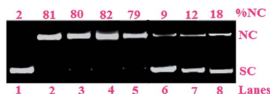
Fig. 5 Photo-induced DNA cleavage activity of complex 2 (100 \mu\text{M} ) in the presence of different additives at 500 nm for an exposure time of 1 h: (lane 1) DNA control; (lane 2) DNA + DMSO (2 \mu\text{L} ) + 2; (lane 3) DNA + KI (0.2 mM) + 2; (lane 4) DNA + catalase (4 U) + 2; (lane 5) DNA + SOD (4 U) + 2; (lane 6) DNA + TEMP (0.2 mM) + 2; (lane 7) DNA + DABCO (0.2 mM) + 2; (lane 8) DNA + \text{NaN}_3 (0.2 mM) + 2.
