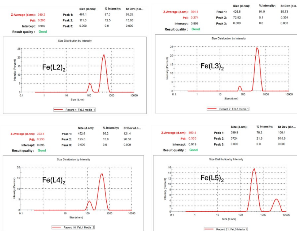
Fig S23: Dynamic Light Scattering (DLS) measurement for Fe(L2) 2 , Fe(L3) 2 , Fe(L4) 2 , and Fe(L5) 2 at 0h and 72 h.
